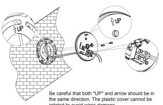
Wires to be pass through the hole of plastic cover. Install the plastic cover to circle crossbar with screws.
